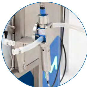
Pre-column instrumentation for conductivity and pH measurement
