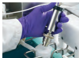
Figure 3. The innovative low dead volume t-connector protects the process fluid from contamination.
