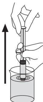
2. Attach the syringe to the Millex® syringe filter.
