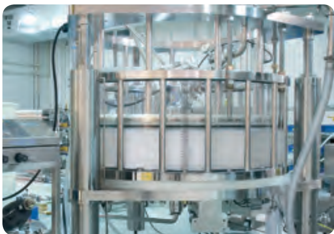
Large-scale column (1.6 m) packed with ProSep® media.
