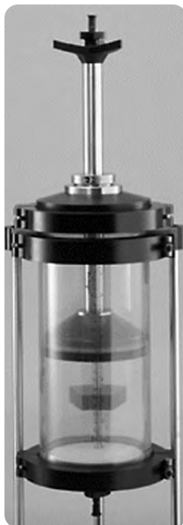
Single action friction lock and fine adjustment assembly.
